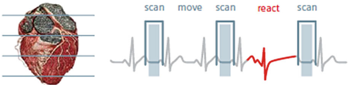
Fig. 15 Each slice of the heart is scanned during the same ECG phase. With this method, substantial dose reductions with no image quality loss are possible
