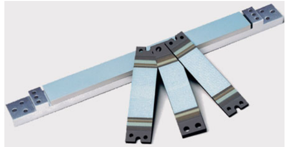
Fig. 5 Multi-detector CT detector modules. Each module consists of rows of detector elements of various sizes. Each module covers 24 channels in the X–Y direction as well as a number of rows in the Z-direction. By combining multiple modules in the X–Y direction, the entire detector array can be constructed
