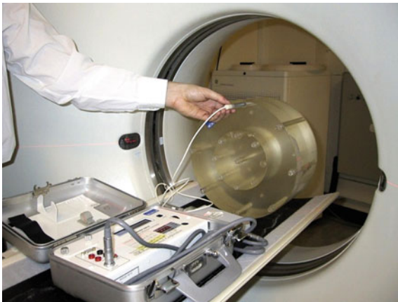
Fig. 1 Standard-sized CTDI PMMA phantoms (14 cm axial length, diameters: 16 head, and 32 cm body), also showing 100 mm ion chamber and electrometer. This body phantom is made up of the head phantom, and an additional annulus to form the body phantom
