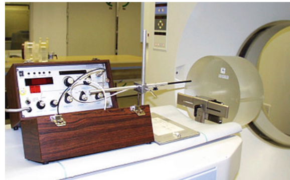
Fig. 12 Ionization chamber and 32 cm lucite phantom used to measure CTDI
