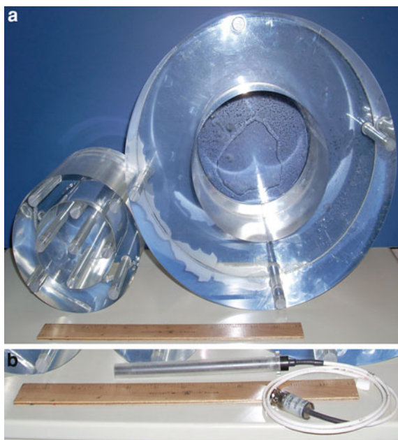
Fig. 3 a Illustrates the two standard CTDI cylindrical plastic phantoms. The smaller cylinder on the left, sometimes called the 'adult head phantom', is 16 cm in diameter. This smaller cylinder is placed in the cylindrical cavity of the larger cylinder shown on the right to create a 32 cm, 'body' cylindrical phantom. b Illustrates the 100 mm long pencil ionization chamber used to measure CTDI doses by inserting it in the holes 1 cm below the surface and at the center of the cylindrical phantoms to make 'surface' and 'central' dose measurements. The ruler shown in both parts of this figure is a standard 12-inch ruler
