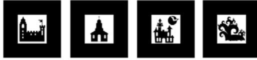
Fig. 5. Fiducial markers used by the system to compute the position of the virtual camera according to the real camera. The marker image is also used to identify the virtual places.
