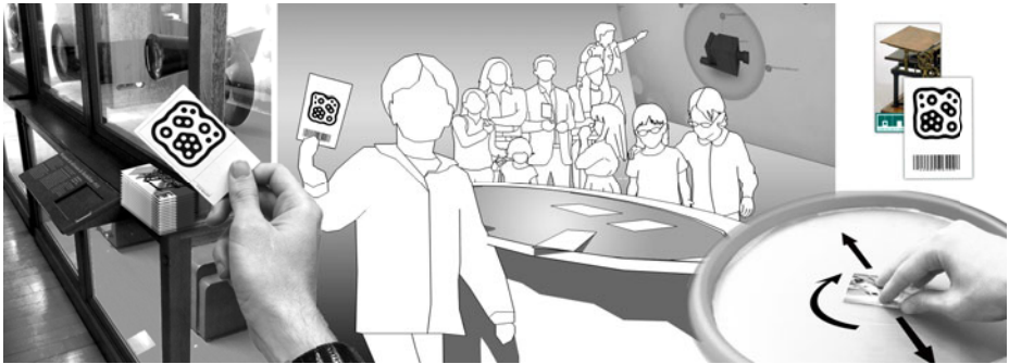
Fig. 1. Paper cards representing object selection. Museum kiosk installation and basic gestures for 3D manipulation.
