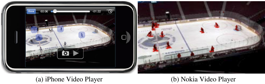
Fig. 2. The iPhone (a) and Nokia (b) rich media players for multi-view video. The iPhone within-video objects are highlighted with relatively large icons for simpler touch access. The Nokia version uses background masks cropped with the annotated bounding boxes to highlight individual objects, which can be selected using the 4-way joystick on the phone.
