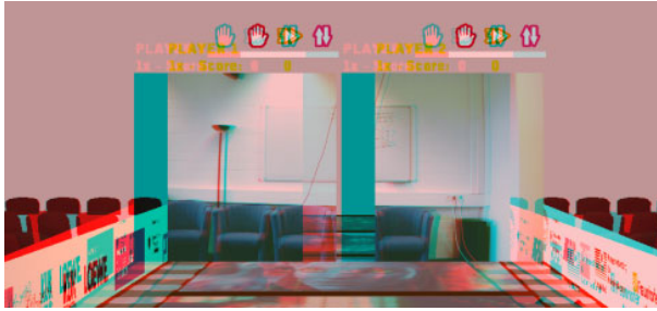
Fig. 3. Occlusion mesh border on two split video canvasses: Since the parallax of the occlusion mesh is adjusted by the 3D Vision driver, but that of the S3D video canvas is not, a black border is perceived by one eye
