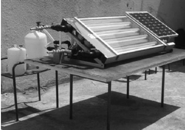
Fig. 16.5 SOLWATER and AQUACAT solar disinfection system [42]
