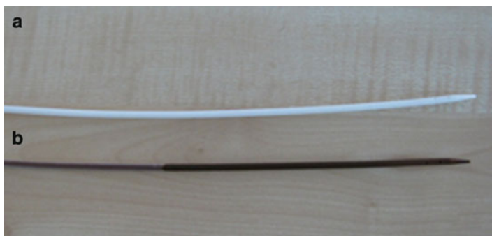
Fig. 11.9 Visual comparison of untreated catheter (a) and silver-treated catheter (b)
