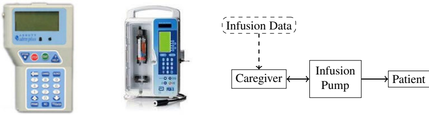
Fig. 2. (left) Examples of commercial infusion pumps and (right) major components of the drug infusion model
