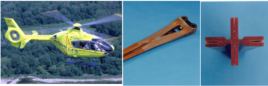
Fig. 1. The commercial EC 135 helicopter with the "flexbeam" main rotor blade structure and the cross section of the torsional element
