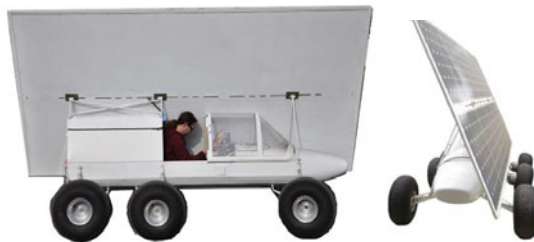
Fig. 3. The Solar Dog, a prototype solar vehicle for an expedition in Antarctica
