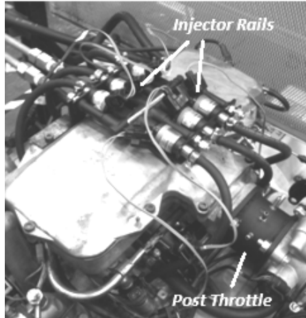
Fig. 1. The GM Holden 3.8lt V6 with the aftermarket CNG fuel system installation
