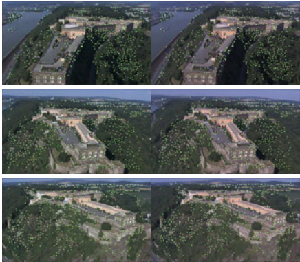
Fig. 10. Stereo frames from the Ehrenbreitstein Fortress sequence. The green dots signify the reprojections of reconstructed 3D points, showing that no drift in the parameters has occurred.
