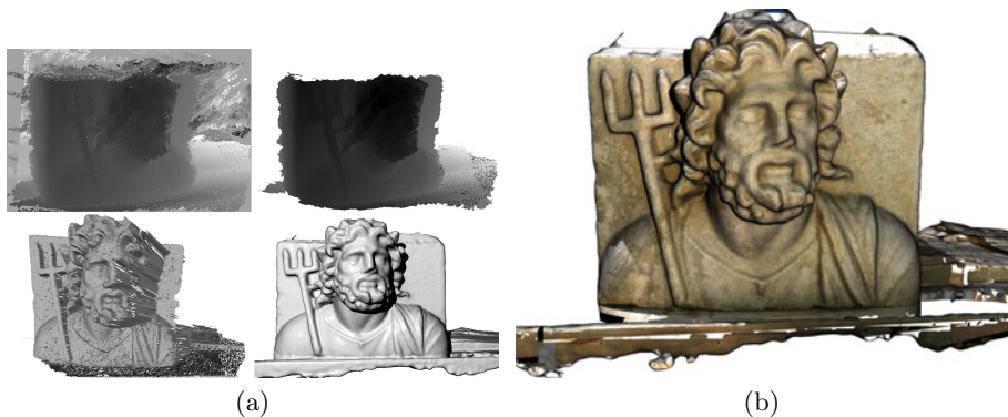
Fig. 3. (a) Creating a mesh out of depth maps. Top left: Original noisy depth map. Top right: The depth map is cleaned and back projected onto a range grid (Bottom left). All range grids are combined and remeshed (bottom right). (b) The mesh is textured to produce the final result. V_{in} = 18 , V_{out} = 4 .
