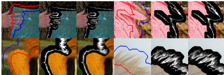
Fig. 5. Example of estimated mixture maps. Each example from left to right: original image with trimap boundaries, \gamma_i before adaptive smoothing, \gamma_i after adaptive smoothing.
