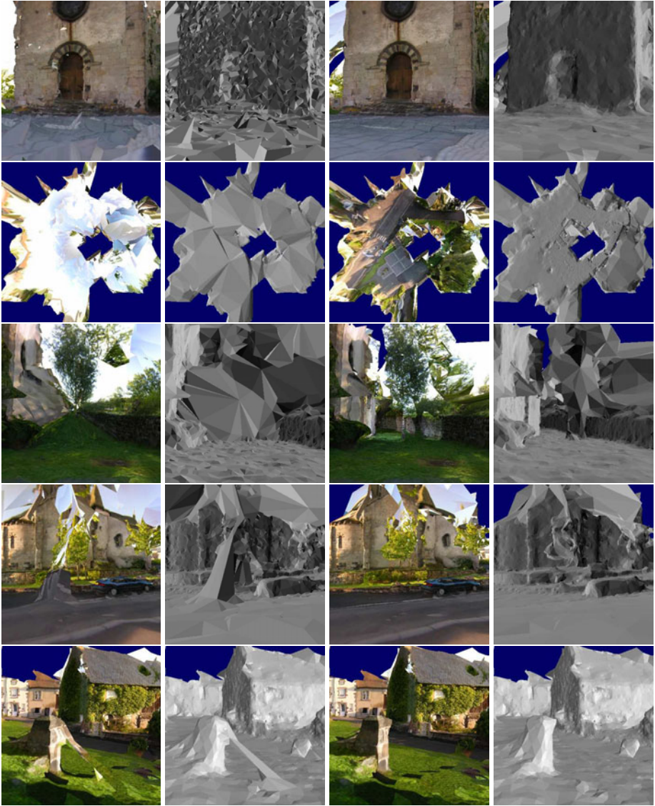
Fig. 5. Row 1: local view of the church 3d model without (left) or with (right) peak removal and surface smoothing (Section 3.5). Row 2: top view without (left) or with (right) the sky removal (Section 3.5). Rows 3 and 4: without (left) or with (right) the “several tetrahedra at once” region growing (Section 3.4). Row 5: without (left) or with (right) the artificial points (Section 3.2). In all cases, gray levels encode the triangle normals.
