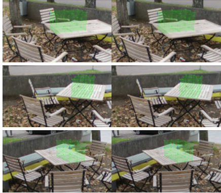
Fig. 9. Real-world sequence shot with a HD camcorder with a 3D conversion lens. The scene has been augmented by a green cuboid to demonstrate the quality of the estimated camera parameters.
