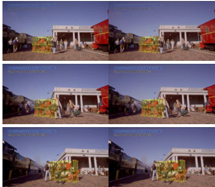
Fig. 11. Stereo frames from the train station sequence. The scene has been augmented by a yellow cuboid to demonstrate the quality of the estimated camera parameters.
