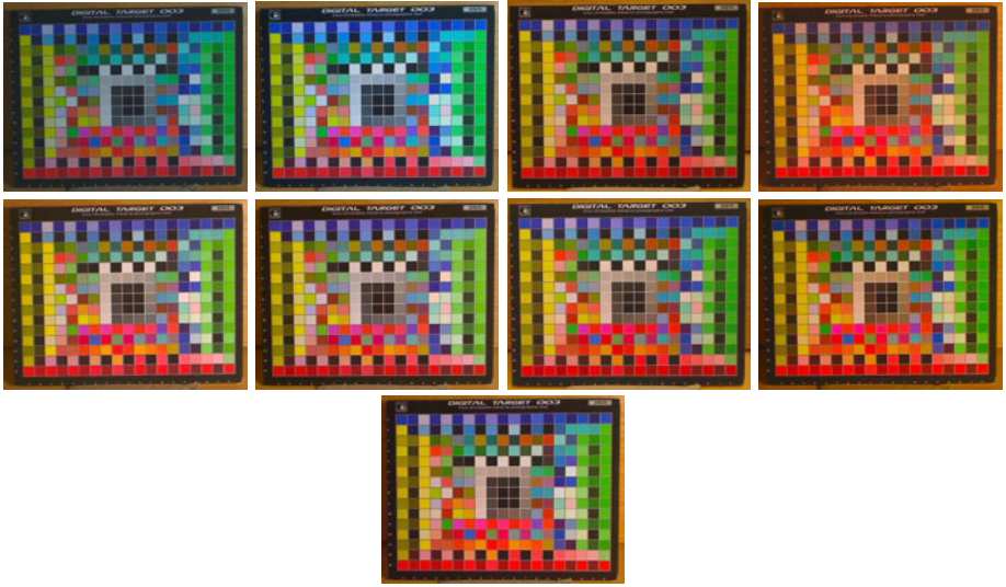
Fig. 4. Appearance of the 285 colour patches with the reference profile applied (top row), and corrected using the corrected profile (centre row) for four different illuminants. For comparison the image taken under the reference illuminant (bottom). The first and third illuminant are less bright, the first and second under slightly “colder” light, the third with a similar colour temperature, and the last slightly “warmer” (also the only incandescent, all others fluorescent).
