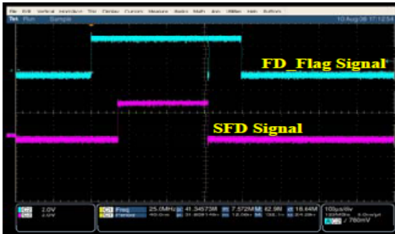
Fig. 11. FD_Flag and SFD when the reception of the first packet was a success
