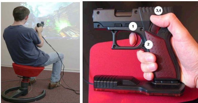
Fig. 3. Advanced input device for FPS: (a) ChairIO and InertiaCube2, (b) PistolMouse device
