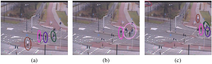
Fig. 2. (a) Tracking before grouping. (b) Tracking during grouping. (c) Tracking after splitting event. The algorithm detects every object and can match all the objects in a correct way.
