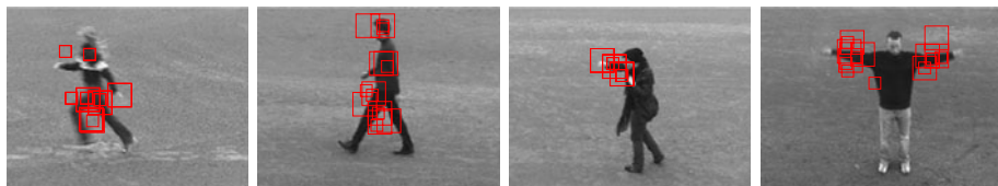
Fig. 4. Examples of space-time interest points extracted at multiple scales for different actions. Clips are taken from the KTH dataset: running, walking, boxing and hand-waving.
