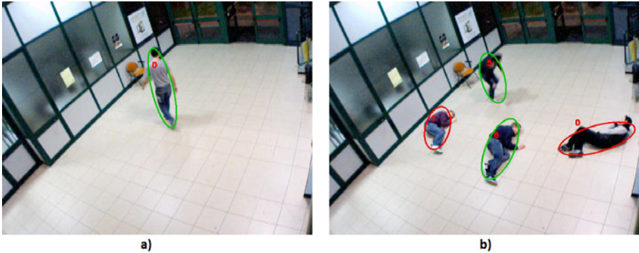
Fig. 4. Excerpts from the dataset; a) simple, single actor scene; b) complex, collective fall. Red ellipses represent already confirmed falls. The third person lying down will soon be tagged as “fallen” too.
