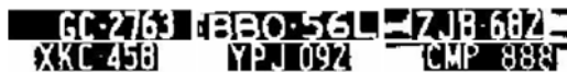
Fig. 5. Binarized images of the images in Figure 3 with upper and lower bounds removed
