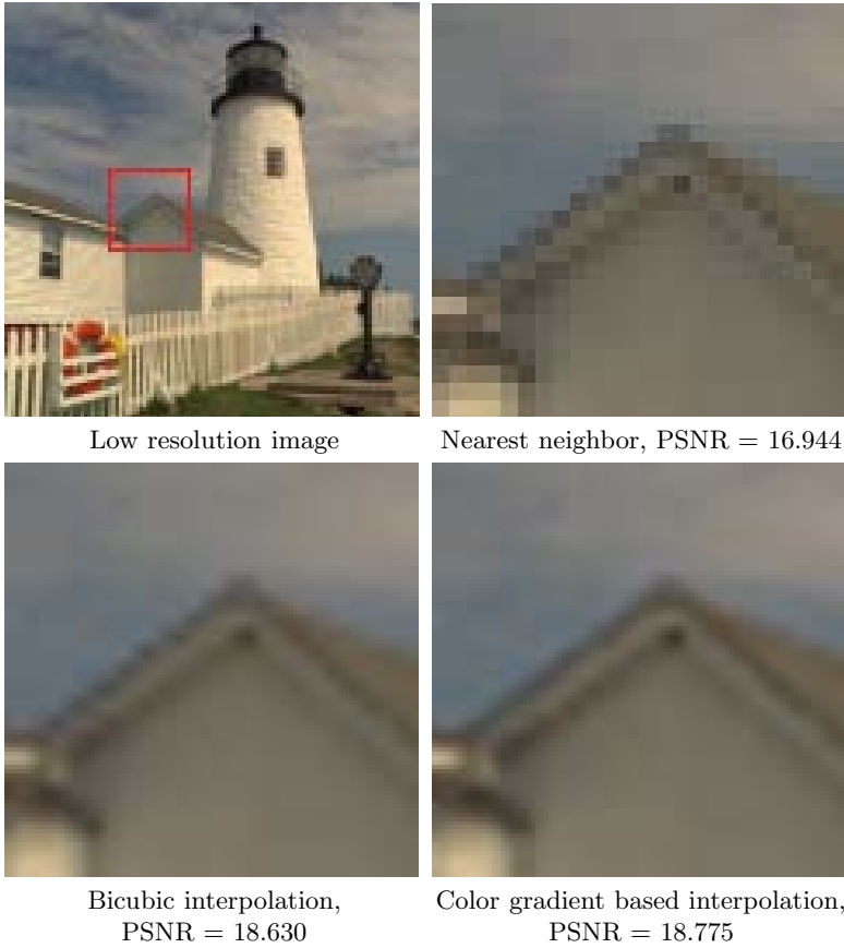
Fig. 2. The results of gradient based 4 times image upsampling for color images with bicubic kernel function
