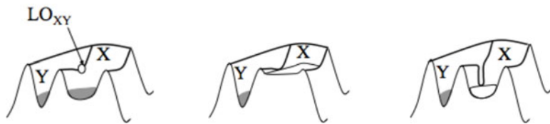
Fig. 2. Local overflow for the catchment basins X and Y. Effect of flooding, middle, and of digging, right.
