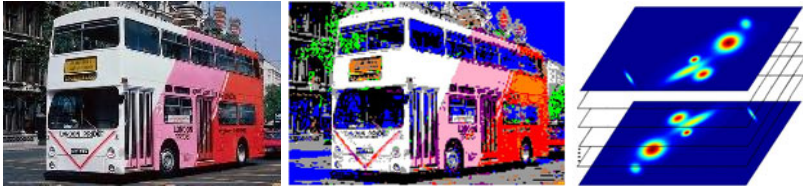
Fig. 2. The construction of the set of GMM models which is a basis for the proposed image retrieval. The original image (left) was subjected to color categorization technique based on FEED model (middle) and each of the spectral images corresponding to 11 basic colors are modeled using GMM approach (right).
