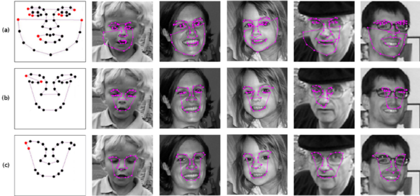
Fig. 2. The three developed models. In leftmost column red points represent the first and last landmark for each shape. Other columns depict examples of features detection. Each row shows the shapes obtained by using the first, second and third face model respectively.
