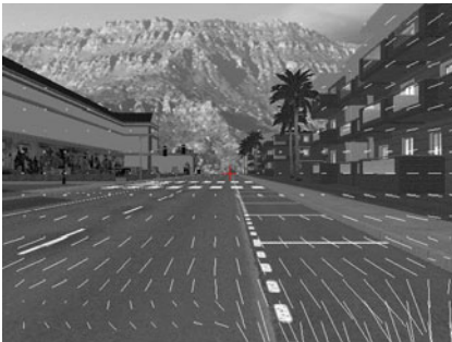
Fig. 6. Image extracted from a Sivic sequence, including the computed Optical Flow and the extracted FoE
