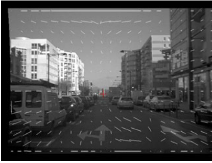
Fig. 8. Image Extracted from a different sequence, including the computed Optical Flow and the extracted FoE
