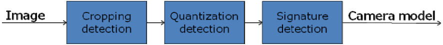
Fig. 1. Block based schema of the pipeline used to retrieve the camera model from an image
