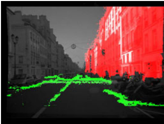
Fig. 2. Image Extracted from a real sequence. Overlays: Red - the building plane ; Green - the road plane.
