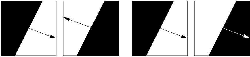
Fig. 1. The edge orientations in (a) and (b) are opposite while their directions shown in (c) and (d) are the same
