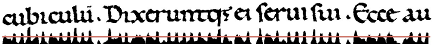
Fig. 1. The number of peaks in the horizontal projection histogram of a row
