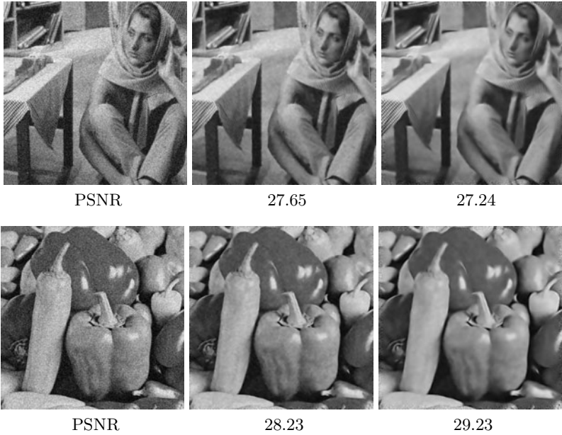
Fig. 2. Image denoising results for Barbara (top) and Pepper (down) images. Left: Image corrupted with 30 std Gaussian noise. Middle: Restored image with kernel size 3 \times 3 . Right: Restored image with kernel size 5 \times 5 . subfigures indicate PSNR values in dB.
