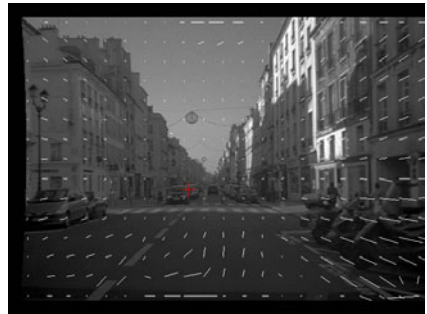
Fig. 7. Image Extracted from a real sequence, including the computed Optical Flow and the extracted FoE
