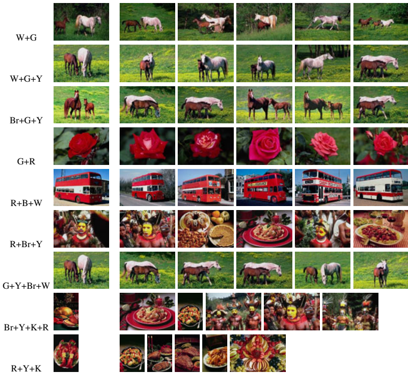
Fig. 5. The results of the retrieval evaluated on the basis of the mixture approximations of a set spectral images corresponding to the colors chosen by user. The experiments tested the efficiency of proposed method for the combination of the following colors, where: white, green, yellow, brown, red, blue and black are denoted by letters W, G, Y, Br, R, B and K.
