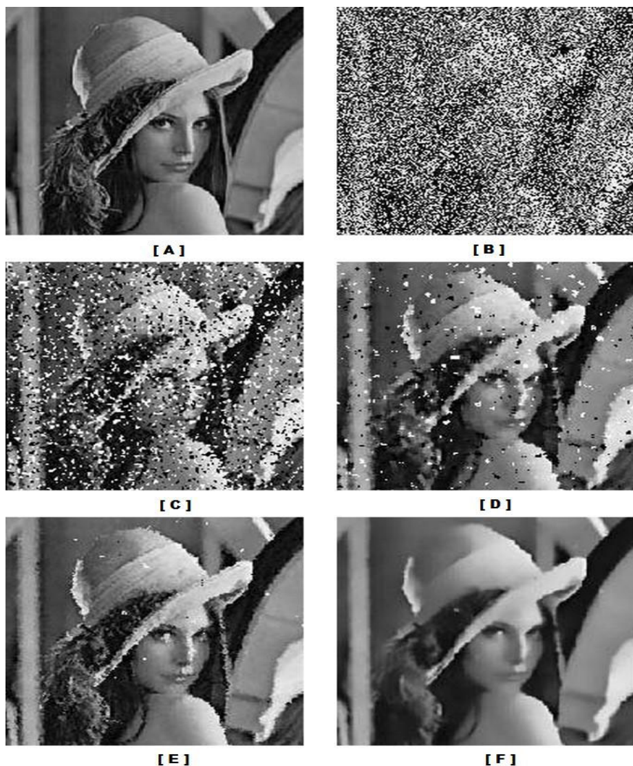
Fig. 4. (A) Original 'Lena.png' image (B) Noisy image with variance-0.6 (C) Median Filter (3x3) output (D) Median Filter (5x5) output (E) Adaptive median filter output (F) Denoised image using proposed method
