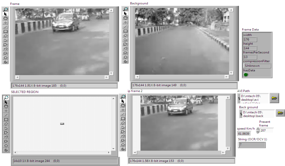
Fig. 10. LabVIEW Front panel for vehicle speed detection
