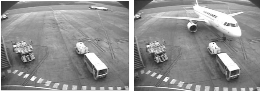
Fig. 4. Snapshots of the ERA (Entrance Restricted Area) after completing Arrival-Preparation. The GPU (Ground Power Unit) is in place. The tanker crossing the ERA in the background (left) causes an erroneous interpretation thread (see text).
