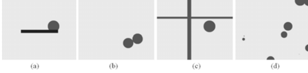
Fig. 2. The synthetic videos used in the comparison. (a): a black rectangle occludes the target; (b): the targets splits into two identical target, then one disappears; (c): a red-shape is in the background; (d) some dots similar to the targets appear and disappear in the background.
