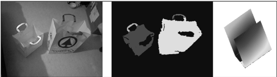
Fig. 2. Left to Right: (a) Input Scene, (b) Detected objects and their corresponding parts in the point cloud (c) Fitting of a cuboid corresponding to the ‘bag’ in the scene
