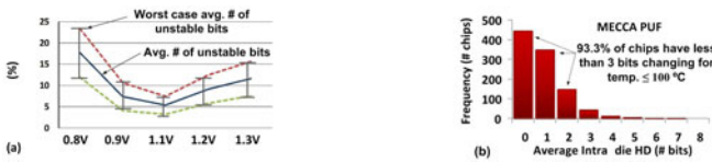
Fig. 8. Average intra-die HD from 1000 chips for MECCA PUF (a) for supply voltage variation (compared to nominal V_{dd}=1V ), and (b) for temperature variation
