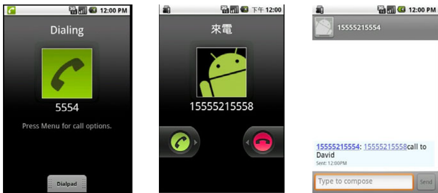
(a) A unknown user calls the user being monitored (b) The user being monitored receives calling from unknown number (c) Call catcher sends the obtained number to monitor via SMS
