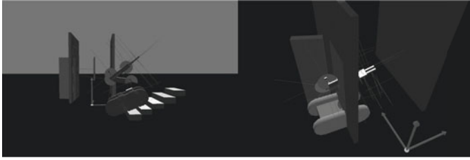
Fig. 9. Left - Climbing the stairs, pitch and roll supervision. Right - Entering opened door.
