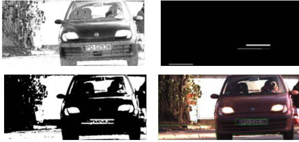
Fig. 2. The process of recognition implemented by the best-of-run individual of WS(P,C) setup: the output of the C filter (top left), the output of the P filter (top right), and the aggregated confidence image produced by the WS aggregator (bottom left), and the final detection outcome (bottom right) with the detected localizations
