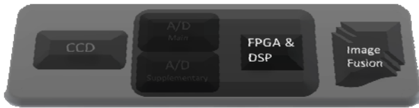
Fig. 2. CCD sensor system with double A/D convertors
