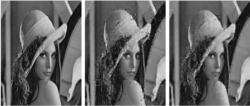
Fig. 3. Block CS Reconstruction ( m/n = 0.4 ). From left to right : (a)lena; (b)original method (PSNR=22.1578); (c)the proposed method(PSNR=25.0346)
