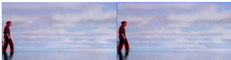
Fig. 3. (a) The initial contour for snake method. (b) The adjusted contour after snake method
