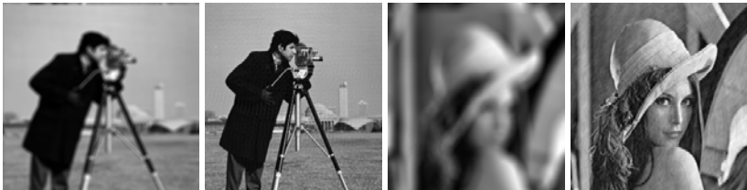
Fig. 6. Out of focus blurred images (left) and their spectral kurtosis based estimates (right)
