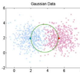
Fig. 3. Allowed concept shift in means of classes, represented by a circular path (green). Means of two classes (red and blue) are marked on the opposite sides of the circle. Artificial recurrence generates datasets with class means distributed uniformly along the circular path, simulating possible drifts in concept.
