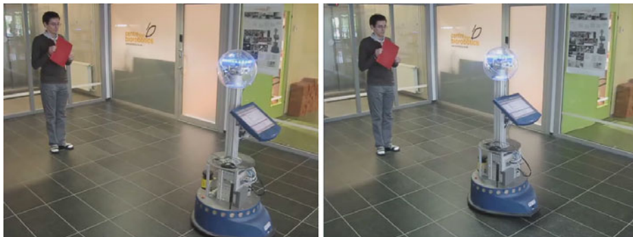
Fig. 3. Robot following a person with a red folder. Robot is moving towards the person, if distance is more than 3 metres (left). Robot stops, when the distance is less than 3 metres (right).
