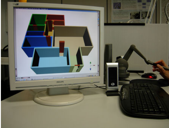
Fig. 2. A multimodal interaction in a VE. The user opens a sliding door with a haptic device. Both the door and the user's haptic probe are controlled with a MIA
