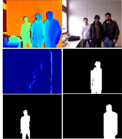
Fig. 4. Foreground object segmentation for Kinect image left to right and top to bottom, original depth image, original RGB image, point cloud projection on the z-x plane (see Block 3 in Fig. 2), object masks for three persons in the scene
