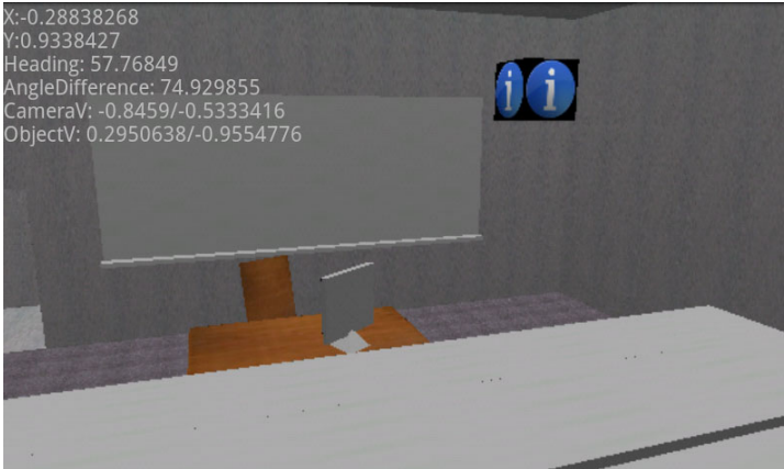
Fig. 4. Screenshot of the application, showing how the virtual camera can match realistic perspectives of a user's position, yaw, pitch and roll
