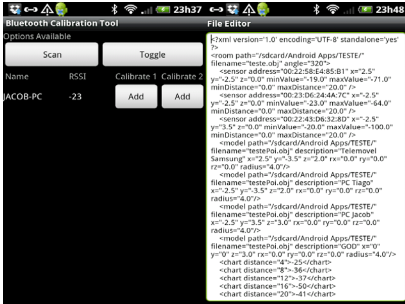
Fig. 3. Screenshot of the calibration tool (on the left) and part of the xml it generates (on the right)
