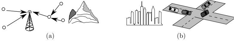
Fig. 6. Examples for wireless networks. (a) Static networks in quasi-static, quasi-free-space environments allow a strong attacker to perform deterministic signal manipulations; we thus confirm the Dolev-Yao model as an appropriate worst-case attacker model. (b) Environments with multipath effects and networks with mobile nodes suggest that deterministic, covert signal manipulations are hard to achieve—a probabilistic attacker model is more realistic.
