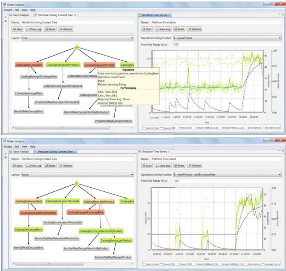
Fig. 3. Kieker screenshots with calling context tree (left) and responsiveness time series (right)
