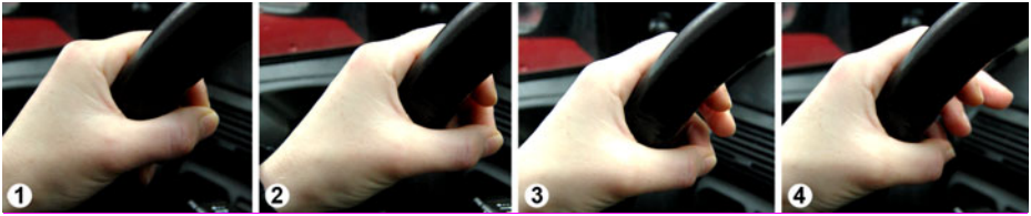
Fig. 5. shows the feasibility of the third gesture of table 1: The thumb can be tapped easily with the middle (2) and the ring finger (3) while holding a steering wheel. But depending on the wheel diameter tapping the thumb with the index (1) or the little finger (4) can be difficult, especially for people with small hands.
