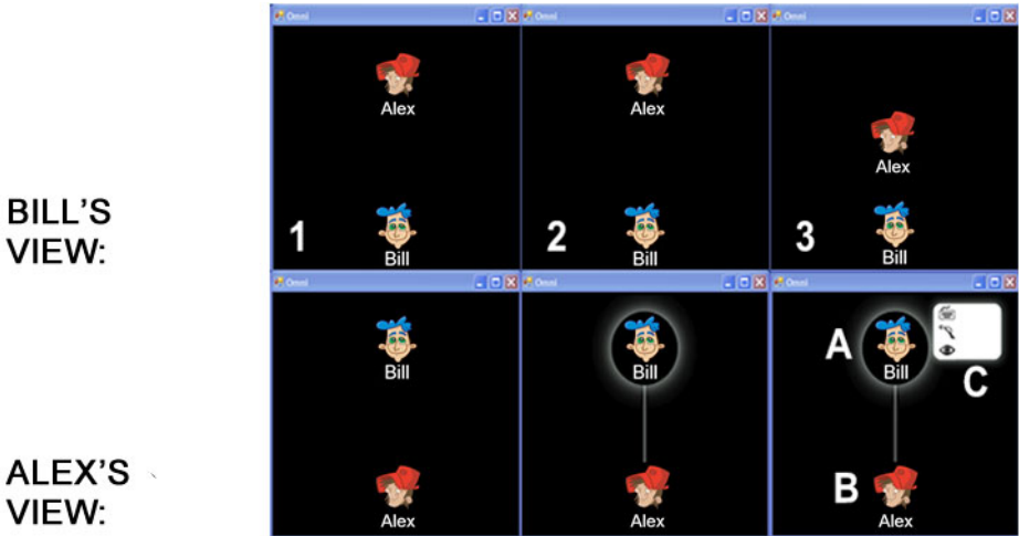
Fig. 2. Screen shots of two OMNI displays in use, with rows denoting what users Alex and Bill see. In Alex’s view, as Alex focuses on Bill, a halo appears around Bill’s avatar along with a line to indicate that he is being focused on. On Bill’s screen Alex moves closer to Bill’s avatar as Alex’s focus level on Bill increases. (A) is the remote user’s avatar, (B) is the local user, and (C) is sensor information about the remote user.
