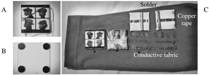
Fig. 2. Patch sensor A) front of final tag B) inner structure of tag showing rare-earth magnets at each corner C) jacket sleeve with conductive fabric; two tags are attached and two tags show circuitry on the back of the tags
