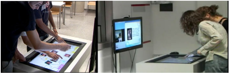
Fig. 1. The system includes two remotely located stations. Participants interact on a horizontal surface while sharing the same workspace with their remote partners. Left ) co-located participants interacting simultaneously. Right ) a vertical screen shows a video feed of the remote location facilitating communication between the two locations.
