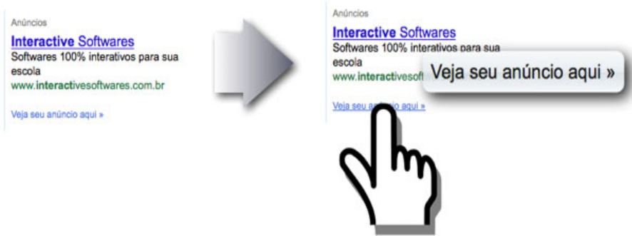
Fig. 1. Outline of the link-offset-scale functionality: as the user positions his finger over a specific link (touching the display), the browser presents the content of that link in a separated magnified element next to the user's finger, so as to be in his field of view
