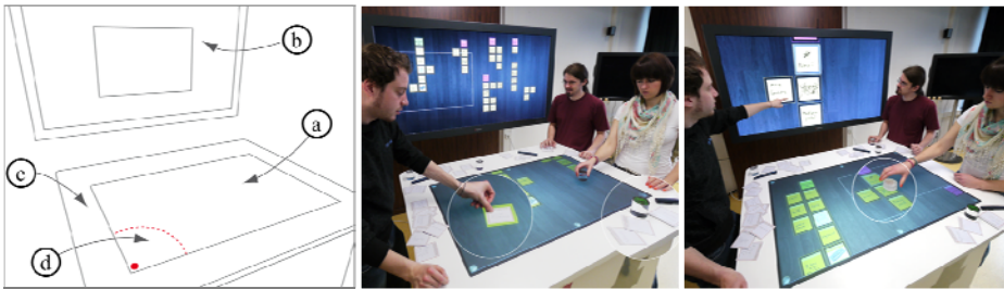
Fig. 2. AffinityTable combines different workspaces by using digital pen & paper, an interactive table with tangible tools and a coupled, high-resolution vertical display
