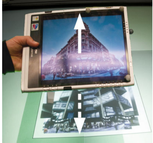
Fig. 5. Browsing stack of photos by holding and moving a tablet computer
