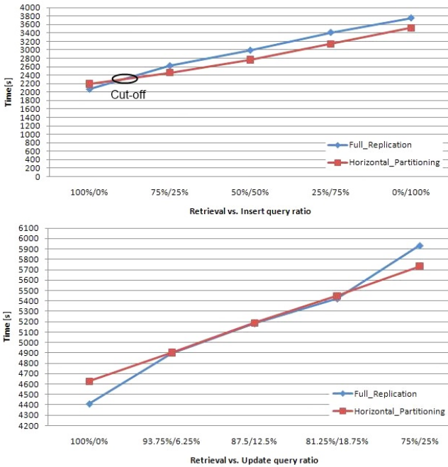
Fig. 2. Cut-off points of Horizontal Partitioning and Full Replication (upper: retrieval vs. insert query ratio with detected Cut-off point; lower: retrieval vs. update query ratio with zoomed Cut-off range)
