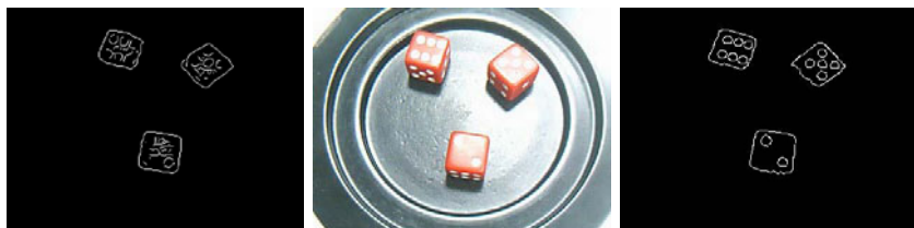
Fig. 1. Middle: specular reflection on the dice; Left: the edge map obtained by previous methods; Right: the edge map obtained by the proposed method
