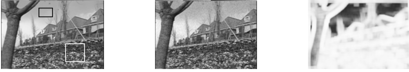
Fig. 3. 40th frame of Flower sequence: black and white rectangles respectively include flat and textured regions ( left ); noisy frame with additive Gaussian noise with variance \sigma^2 = 225 ( middle ); point-wise SSIM index between original and noisy frame ( right ).
