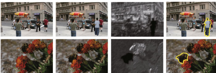
Fig. 5. Shown above are the results of local tamper detection. The first column shows the original images. The second column shows the tampered images. Column 3 shows the calculated R map. The final results are demonstrated in column 4. The boundaries of the tampered region are highlighted.
