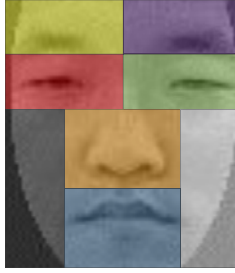
Fig. 1. Eight face patches illustration. Left eyebrow(yellow), left eye(red), left cheek(black), nose(orange), mouth(blue), right eyebrow(purple), right eye(green), right cheek(white).
