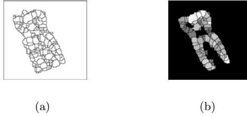
Fig. 2. Results of consecutive stages of the algorithm: 2(a) watershed segmentation, 2(b) regions remaining after thresholding, with brightness equal to their fitness value
