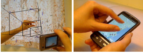
Fig. 1. 3D interaction vs. 2D interaction. Left: User capability to move in depth and change the finger size according to the distance to the camera. Right: Limited area for user's fingers in 2D interaction.
