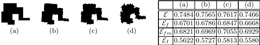
Fig. 1. Shapes with a different noise level added and their corresponded \mathcal{E} , \mathcal{E}_f , \mathcal{E}_{fm} , and \mathcal{E}_I values
