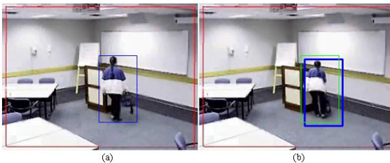
Fig. 4. Example of applying location smoothing algorithm. (a) Original patch (b) New location is indicated by the green bounding box
