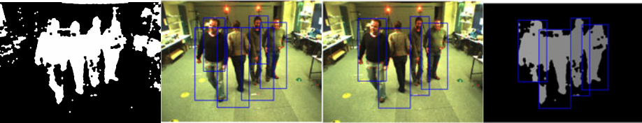
(c) From the final disparity map, different depth of the persons can be observed
