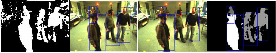
(a) Multiple candidates on one person have been merged due to similar depth
