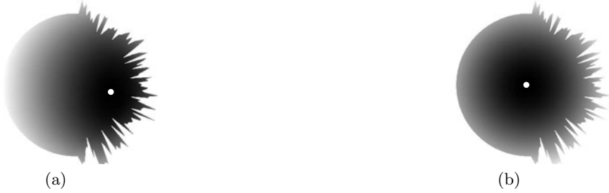
Fig. 1. Centres determined by minimising the geodesic distances to (a) the shape boundary, (b) the shape interior. The geodesic distances to the centres are displayed inside the shapes.
