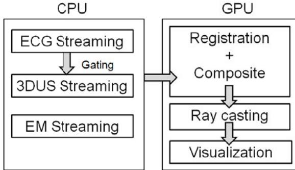
**Fig. 1.** Data flow between CPU and GPU
