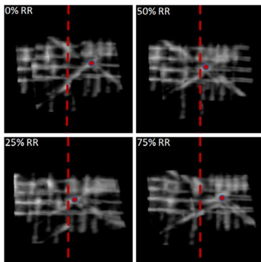
**Fig. 5.** Mosaiced results at different RR intervals. The red dot is the fiducial point on the string phantom. The red dotted line indicates the mid line of the cross section. The varying distance between the fiducial point and the mid line is the result of the motion of the phantom.
