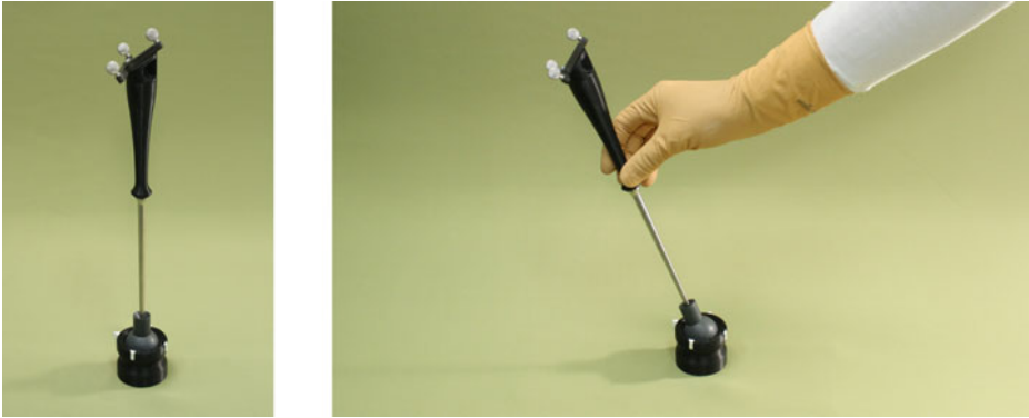
Fig. 1. The input device is activated when a tracked surgical probe is inserted into the base. Force feedback returns the probe to center and permits clicking.
