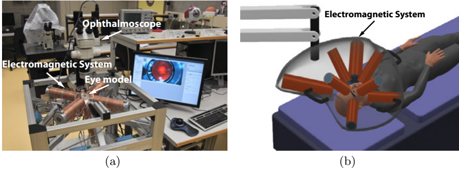
Fig. 3. (a) The OctoMag electromagnetic control system with an eye model in its workspace, and (b) rendering of a future system for AMD treatment
