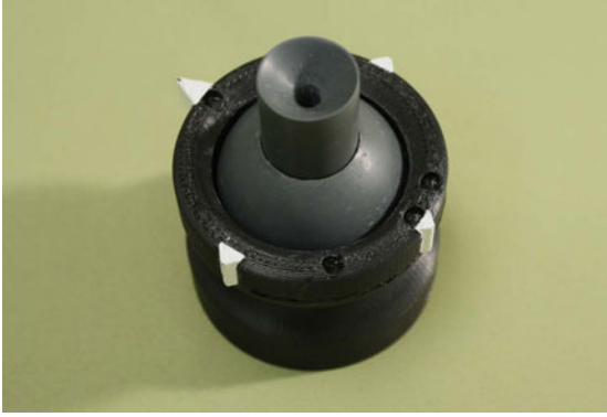
Fig. 2. The base of the joystick device. The probe is inserted into the hole on top of the small cylinder and can be tilted with two degrees of freedom. Pressing the probe down to click causes the small cylinder to move into the ball while still permitting the probe to be tilted.
