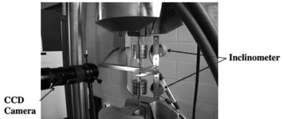
Fig. 20 DCB specimen in the testing machine with inclinometers attached to the adherends and camera for measurement of \theta and \delta_n , respectively (Ji et al. 2010)
