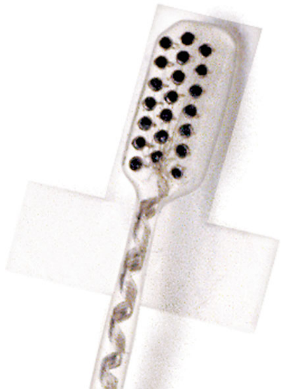
Auditory Brainstem Implant, Surgical Devices, Fig. 2 Close-up of electrode array of auditory brainstem implant (Image Courtesy of Cochlear Americas ©2011)
