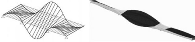
Fig. 3. 4 th mode shape 2.09 Hz (measurement) and 2.29 Hz (calculation) – 1TL main span [17]
