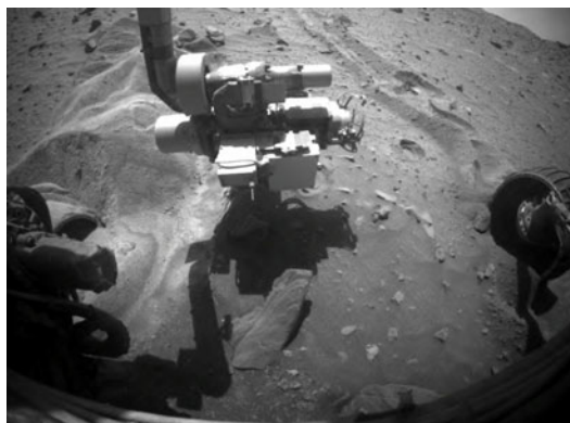
Fig. 1. Spirit Rover showing front left wheel stuck in soft soil in location ‘Troy’(Source: NASA)
