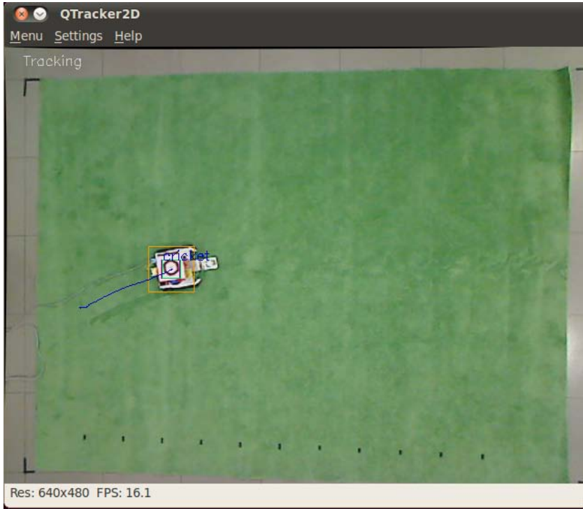
Fig. 5. The robot is automatically tracked using an overhead camera and custom-built tracking software [1]
