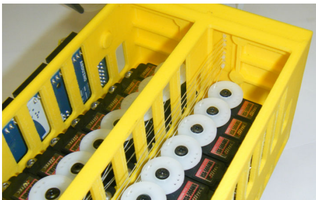
Fig. 6. The actuator housing that encloses the actuators and associated hardware. The servomotors can be seen mounted in 1.5 mm vertical steps aligned with the actuator tendons.
