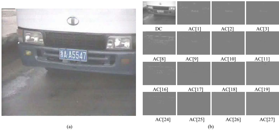
Fig. 1. Feature extraction from DCT coefficients. (a)768×512 input image (b)DCT feature from the intensity image.
