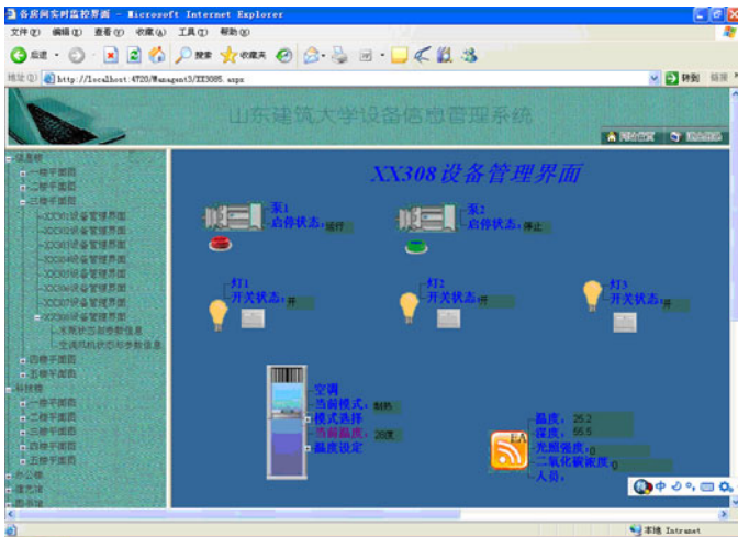
Fig. 4. Interface of Equipment Management System
