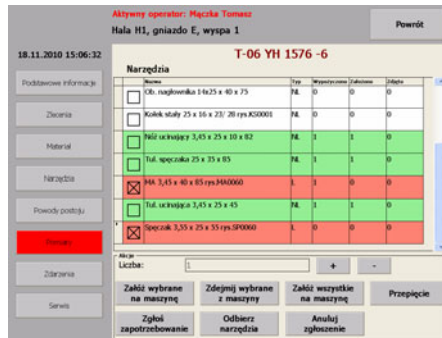
Fig. 13 Shop-floor main HSI screen for the tools-management module
