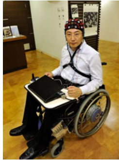
Fig. 7 Toyota wheelchair controlled by BCI [Toyota 2009]
