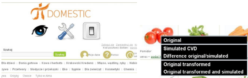
Fig. 1 The main web proxy menu (left) and an image transformation menu (right) of the proxy (examples use the web site of the Polish online shop: www.alma24.pl ). Colorful images for all figures are available in the electronic version of this paper
