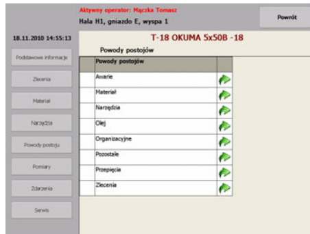
Fig. 10 Shop-floor HSI unlocked mode screen for stop reason data inputting
