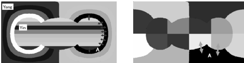
Fig. 2. Schematic features of domain decomposition on Yin-Yang grid system. Left: one dimensional domain decomposition, and Right: two dimensional domain decomposition.
