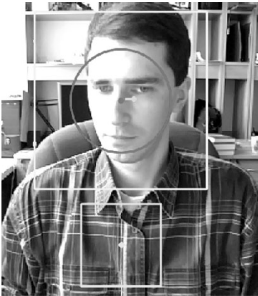
Fig. 4. Illustration of the head gestures detection algorithm: circle with center dot—current face position, not centered dot—the reference face position, dash—head movement vector, large square—face finding region, small square—the region for body movement detection
