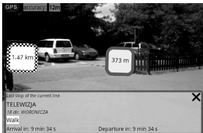
Fig. 1 Augmented reality view generated by the NavAR application. The right marker indicates the position of the last stop of the current line and the left marker indicates the position of the destination location
