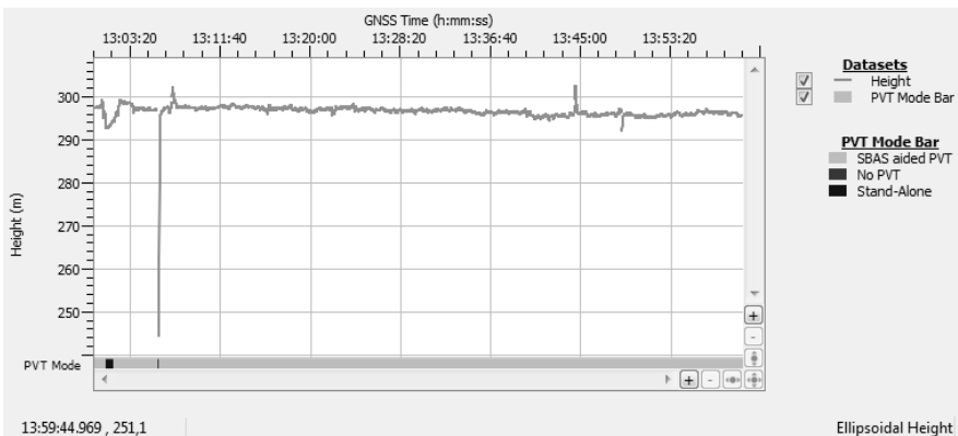
Fig. 7 Integrity Event 338—impact on the Height Position
