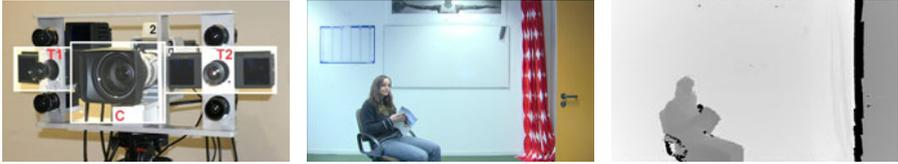
**Fig. 1.** From left to right: Camera setup, color image from central camera  $C$ , warped depth image from cameras  $T_1, T_2$
