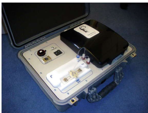
Fig. 11 Top: Integrated smart RNA hybridization sensor composed of sensing unit, preconcentration unit, and dehybridization unit. Bottom: A functioning prototype measuring 25 \times 10 \times 40 cm is shown in which a glass chip (like that shown in Fig. 10 but containing the multitarget design) is seen at the top of the instrumentation. A handheld prototype is expected in a year
