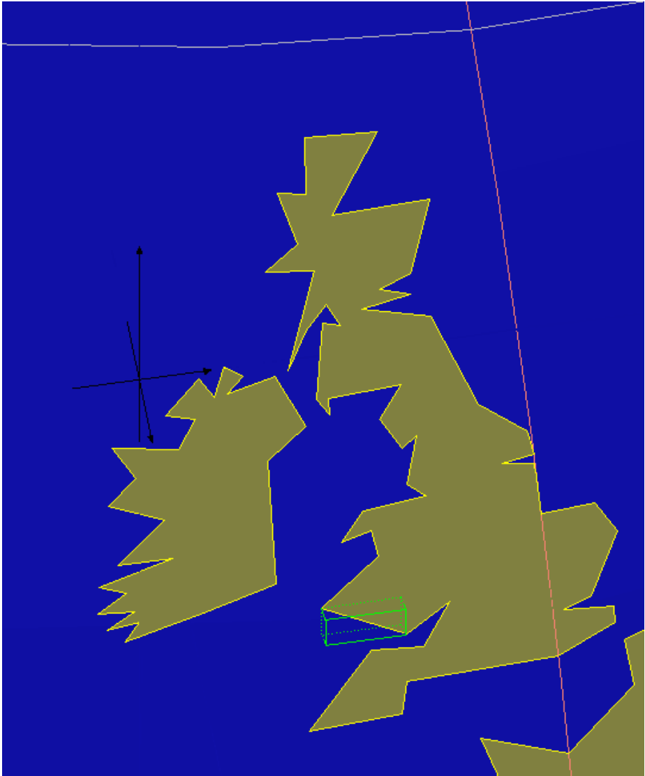
Fig. 1. A simplified version of Great Britain: The pink line is the Prime Meridian and the white line has a latitude 60^\circ north. Three axes in black have their origins at the center of the Earth. The 3D MBB (in green) is obtained from a line segment of Great Britain. Some green lines are dotted because they are under the Earth's surface.
