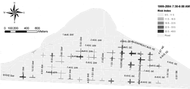
Fig. 8. Result from the map generator – risk map of morning rush hour (7:30-9:00AM) of Calgary downtown area
