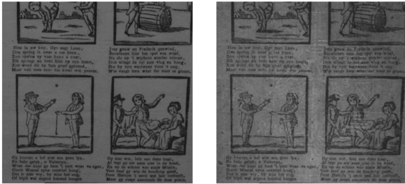
Fig. 2 Reflection-transmission (left, front and back illumination) and transmission (right, back illumination) infrared data images of a document printed on watermarked paper
