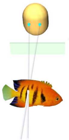
Fig. 1. Our virtual robot, Emer. His name is based on “emergent”, our neural network simulator. Seen here are his torso, head, eyes, eye-beams, and the fish that he is foveating in preparation for object recognition. Emer is implemented using the Open Dynamics Engine rigid body physics simulator [6] and the Coin3D 3D Graphics Developer Kit [4]. Each of his eyes is a camera, and their offset positions on his head give him slightly different views of objects, facilitating stereo vision.
