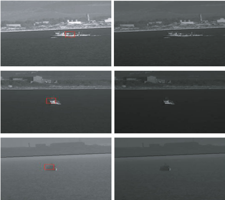
Fig. 10 Real-time Video Algorithm Performance: Real video camera on USV in different light and sea states and targets radius. Selected movies can be found on-line at [13].
