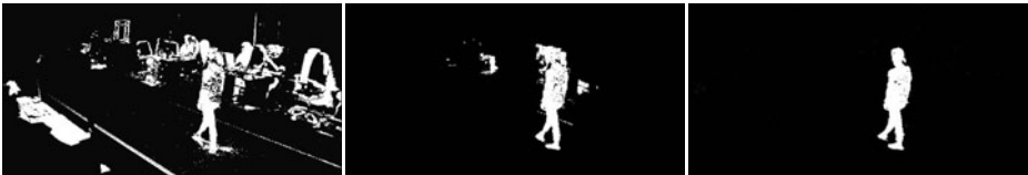
Fig. 3. First image of test sequence, from left to right: 1. Difference between input foreground and background images (binary threshold), 2. Proposed algorithm after one iteration without spatio-temporal optimization (gray values correspond to inferred probabilities), 3. Result of proposed algorithm with spatio-temporal optimization after two iterations
