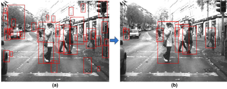
Fig. 5. Cascading distinct classifiers with two heterogeneous features. (a) Extract possible pedestrian candidates by simple joint Haar-like features. (b) Verify each candidate by high dimensional CoHOG descriptors.
