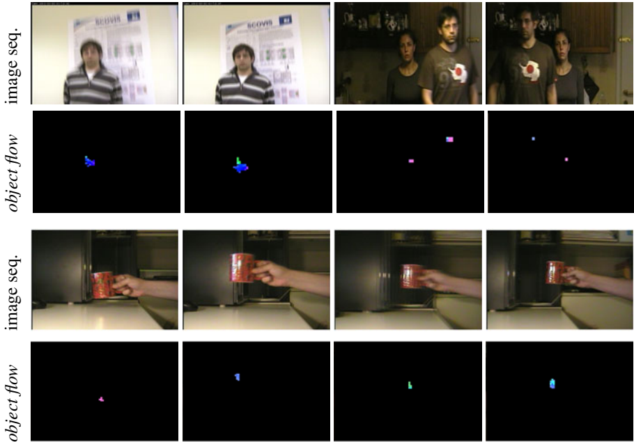
Fig. 7. In this experiment we train the classifier to deliver Object Flow for different object classes including faces and a coffee mug. The first and third row depict frames from different test sequences (camera movement, motion blur and multiple objects). The second and fourth row present the estimated Object Flow , respectively. (Video is available at the authors' web-page.)
