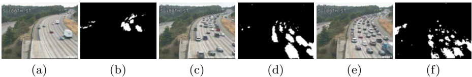
Fig. 3. Light, medium and heavy traffic. The connected components of the active regions increase as the traffic gets heavier.
