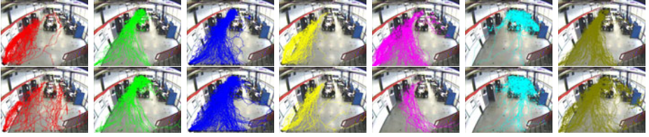
Fig. 2. Top row: the 7 estimated common behaviors from the initialization phase. Below: clusters induced by the association of test data.
